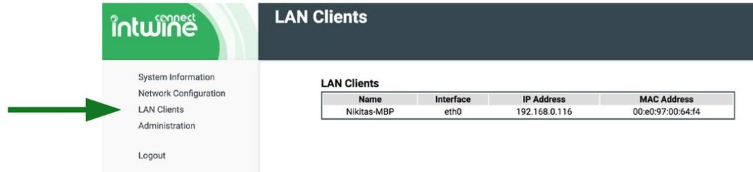
The **LAN Clients** tab shows a complete listing of all WiFi and/or Ethernet devices that are connected to the gateway. Each LAN client will show its **Interface** (WiFi/Ethernet), **IP Address**, **MAC Address**, and for devices that have been assigned a **Name**, that will show as well.
