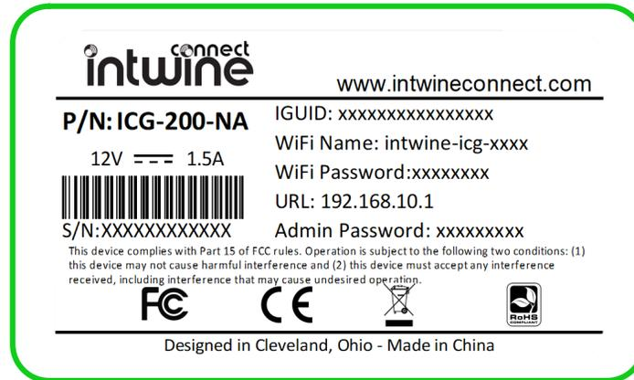
A variant of the above pictured label ships on every production ICG-200 with both standard information and information that is specific to each individual Gateway. The label is full of pertinent information including the router's FCC ID, UL number, MAC address, serial numbers, etc. The three most important pieces of information for configuring the ICG-200 are labeled above and described below:
