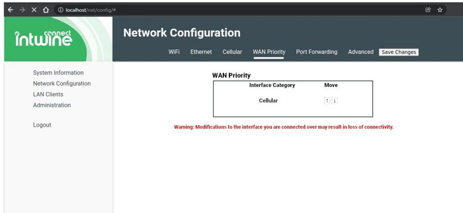
Allows users to choose primary and secondary WAN connections. For example, in a typical cellular backup scenario, a user will want to configure Ethernet as the Primary WAN (priority 1) and Cellular as the backup WAN (priority 2), in case of a network outage.
