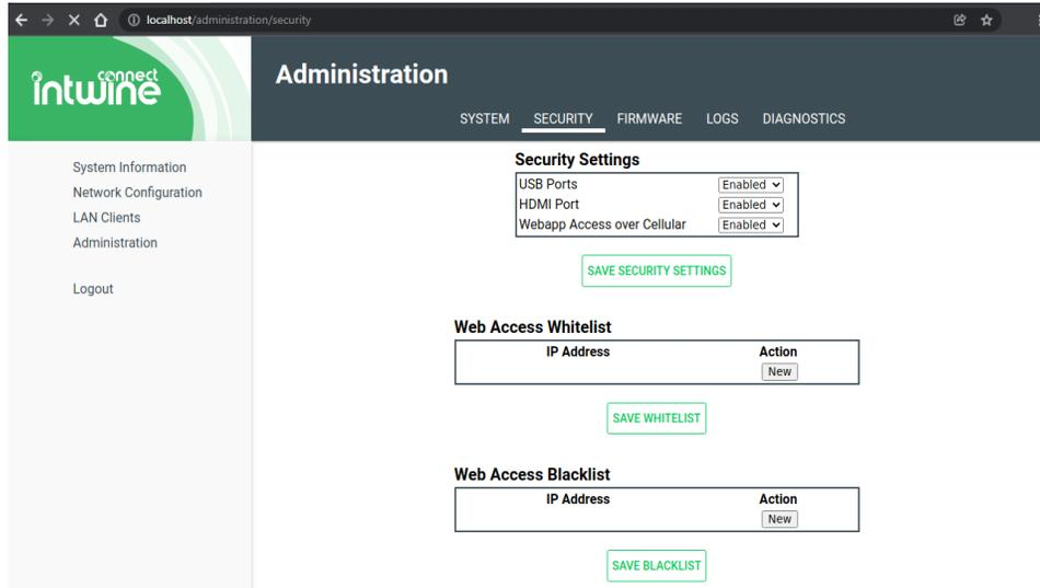
The page also allows you to allow or block specific IP addresses from accessing the local configuration webapp. The ICG-200 will automatically detect remote intrusion attempts and block those devices without any user intervention.
