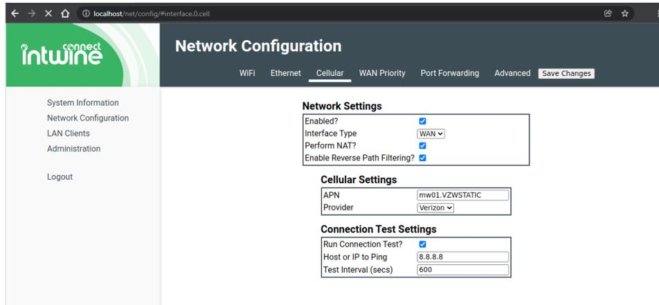
The **Cellular** tab allows users to configure which interfaces are configured as **WAN/LAN**. The **APN** and the **Provider** can be changed.
