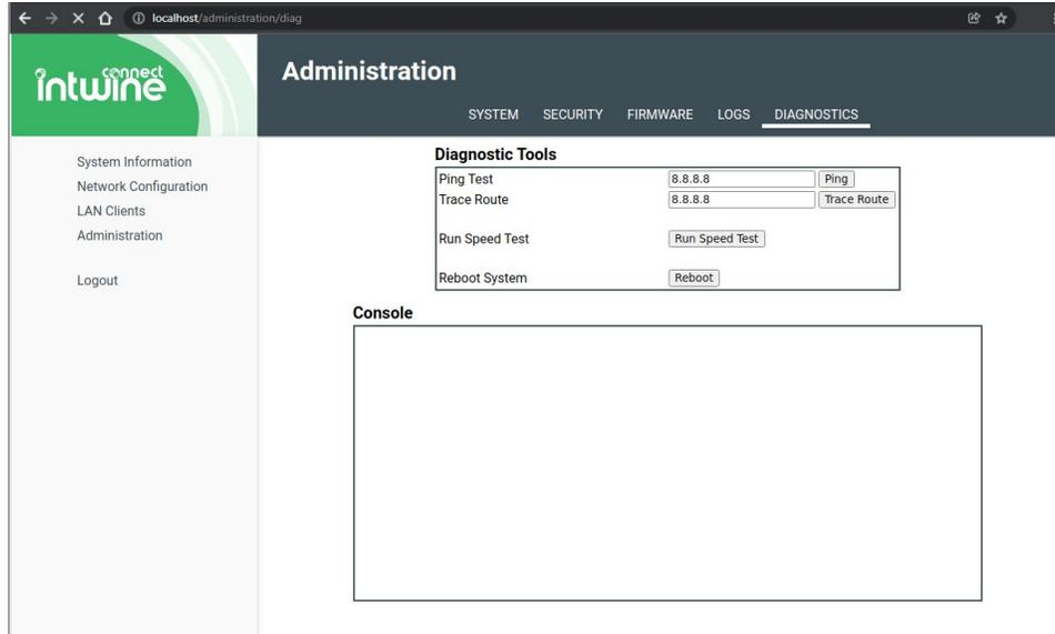
The **Diagnostics** tab allows users to conduct tests to help determine that their system is properly working or to isolate and resolve problems. Users can make the ICG-200 ping a specific IP address or URL as well as run a trace route. These tests can allow you to resolve network connectivity problems. Users can also have the system run a speed test and reboot the system.
