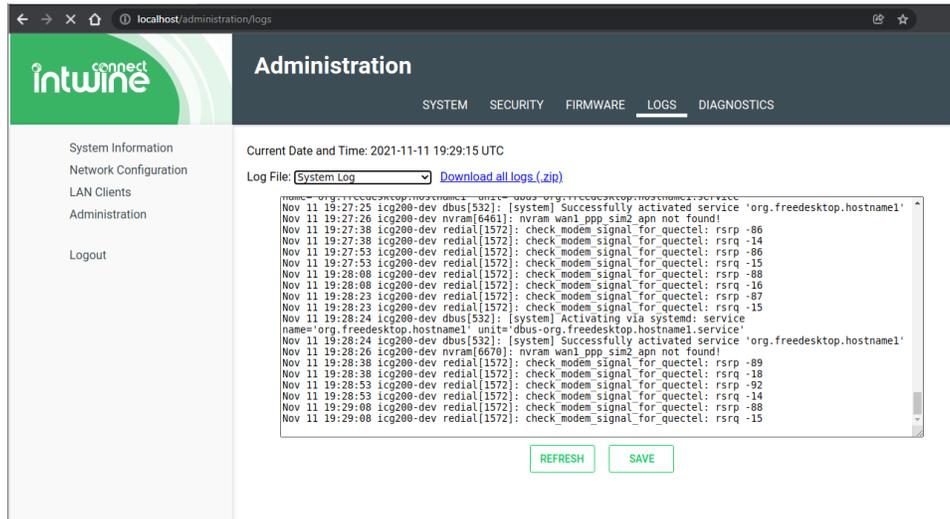
The **Logs** tab allows users to take a look at or download the logs. The available log files are – **System Log, Application Framework, Network Config daemon, ICG Log.**
